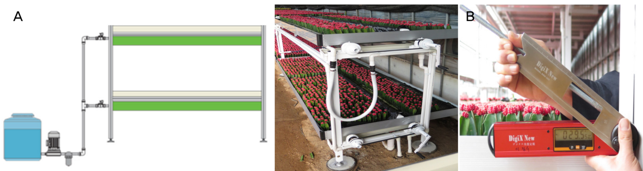
Fig. 2. Ebb-and-flow hydroponic system with double-tier bench for grafted cactus: appearance of hydroponic bench (A), and bench backside of incident angle on sun (B).
